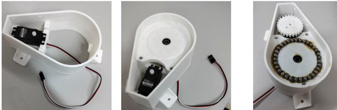
(a) Attaching the servo motor to the base support, enabling base rotation. (b) Installing the main gear in- drive rotation. (c) Adding the lower gear, and pulley to enable smooth base rotation.
